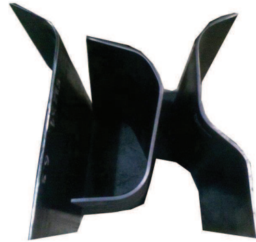
Bended samples (500x500 mm) in 4 and 5 mm thickness
