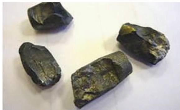
Projectiles cores destroyed by Mars® 600 hardness
